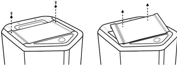
3. Remove the battery using the pull tabs.
