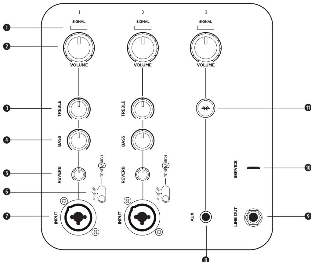
Use Channel 1 and 2 inputs for microphones and musical instruments. Integrated ToneMatch® signal processing allows microphones and instruments to sound their best. Use Channel 3 for *Bluetooth*® connectivity and line-level inputs.
