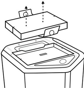
4. Insert the new battery, ensuring the connector pins line up appropriately.
