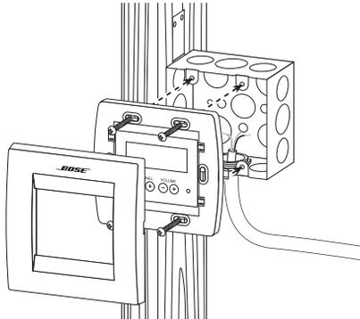
After screwing the frame into the wall box, remove the protective clear film and snap on the cover. The cover can be removed later using a small flathead screwdriver in the slots on the sides.
