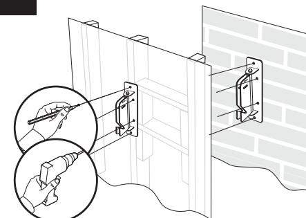
Minimum Installation Requirements when mounted to wood studs:  $\frac{1}{4}'' \times 1\frac{1}{2}''$  (M6 × 38 mm) lag screw
