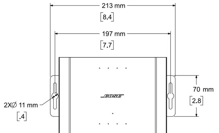
1. DIMENSIONS ARE SHOWN IN MILLIMETERS OVER INCHES.
