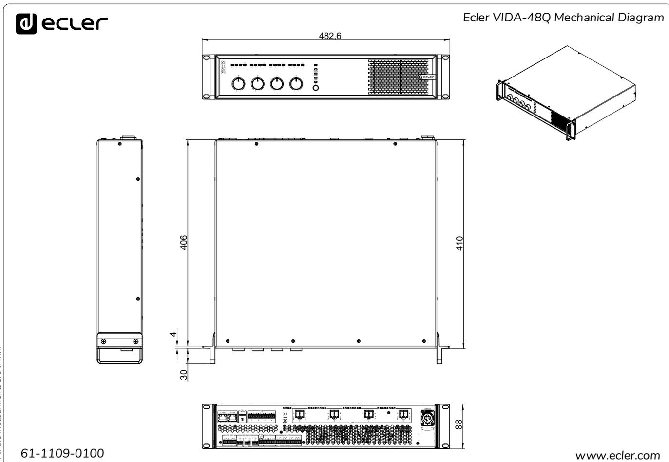
All the measurements are in mm
