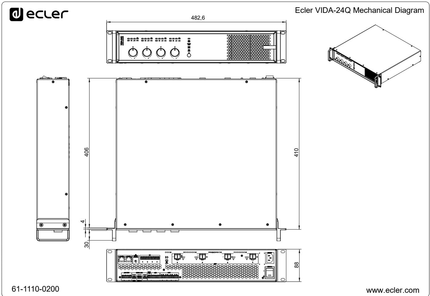
All the measurements are in mm.
