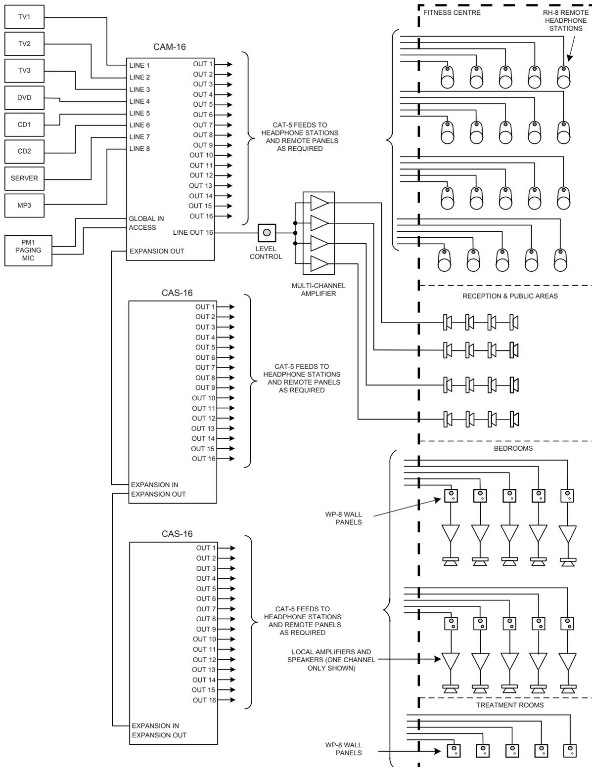
The example shown uses a CAM-16 distribution matrix and two CAS-16 expansion units to produce a total of 48 outputs. Each of these may be routed to an RH-8 remote headphone station or a WP-8 wall panel as required, anywhere in the building. Each RH-8/WP-8 will have individual selection of audio source and volume control.
