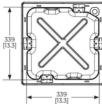
8. Dimensions are shown in millimeters over inches.
